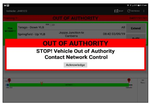
The Out-of-Authority condition will only be triggered if the rail track vehicle is not within any of the TOA's it is associated with. Once acknowledged, the Out of Authority alarm banner remains at the top of the display until it is no longer a valid alert see below.
