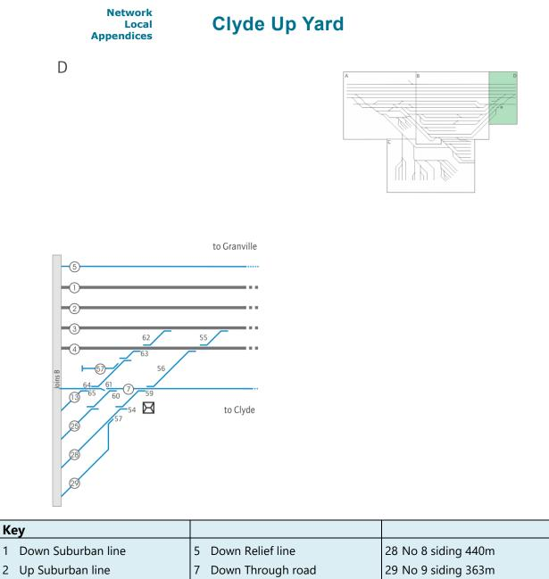
1Down Suburban line5Down Relief line28No 8 siding 440m2Up Suburban line7Down Through road29No 9 siding 363m3Down Main line13No 5Reception siding 490m57Storage siding 173m4Up Main line25No 4Grid siding 458m57Storage siding 173m
