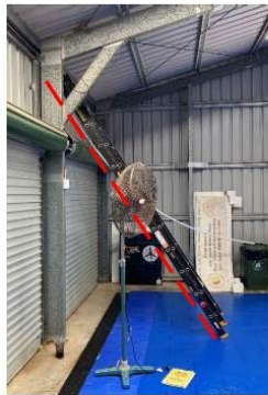
Incident scene re-enacted. Note: Ladder could not be installed at required 4:1 slope due to its length.
