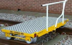
Photos: Example of Rail Push Trollies in tare condition indicating the GVM up to 1250kg.
