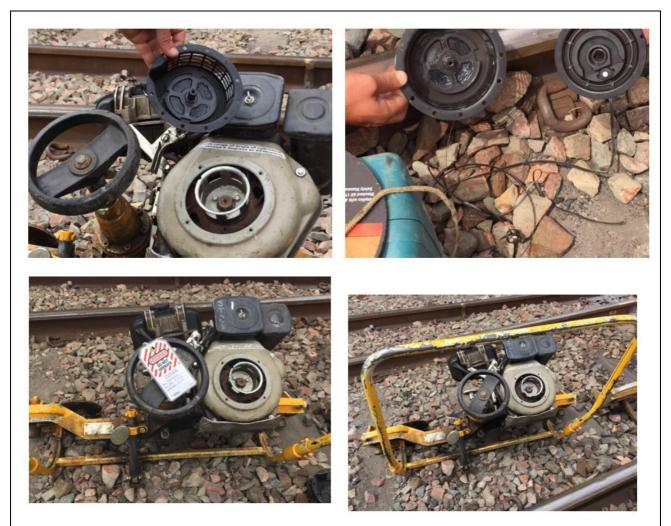
Separate unit shown below with pull cord and cover in place.
